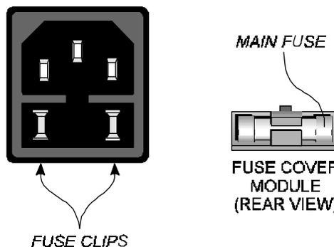
After replacing the fuse with another of identical specifications, push the fuse cover module fully back into place, ensuring that the fuse has snapped onto the fuse holder inside the power inlet module.
