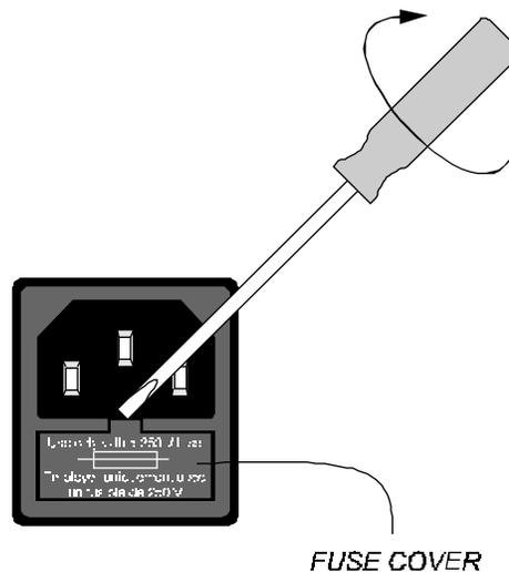
Use a small flat screwdriver as shown to slide the fuse cover out from the power inlet module. The fuse can be found inside the fuse cover module after it is pulled out.
